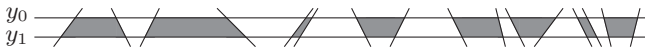
Figure 13: The intersection of polygon A with the horizontal slab [y_1 : y_0] consists of a set of trapezoids.
