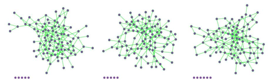
Three realizations of a random network with p=0.03 and N=100. Several nodes have degree k=0, shown as isolated nodes at the bottom.
